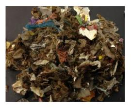
Scientific literature and experience have shown that waste moisture heavily compromises the final quality of the alternative fuel and keeps its calorific value low.
